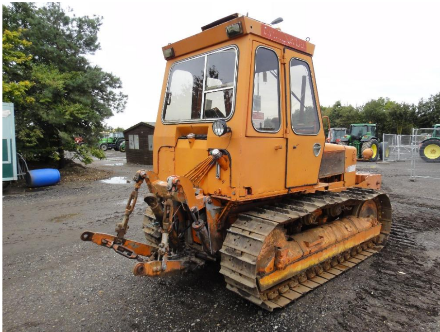
Gambar 6. Traktor beroda track/crawler logam
