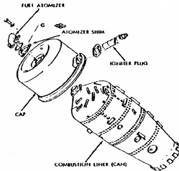
Gambar 13 Combustion chamber jenis can
