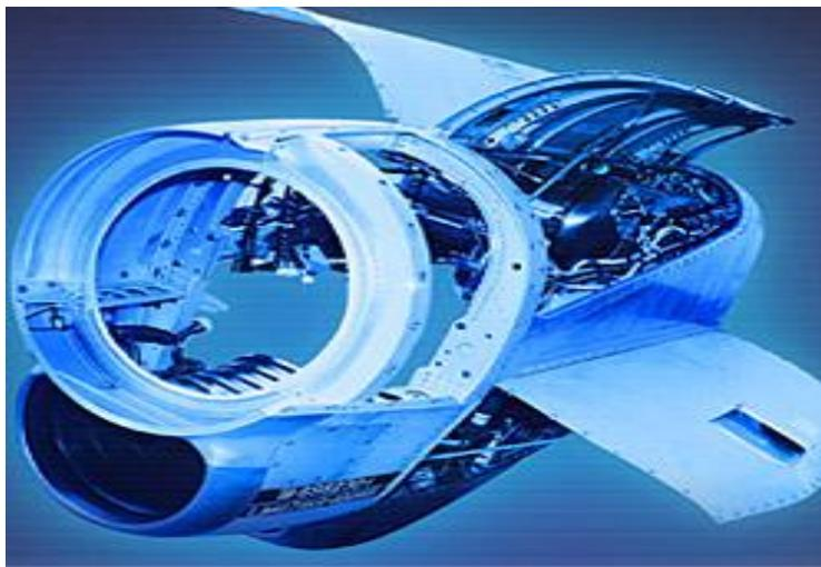
Gambar 28. Bukaan engine cowling
