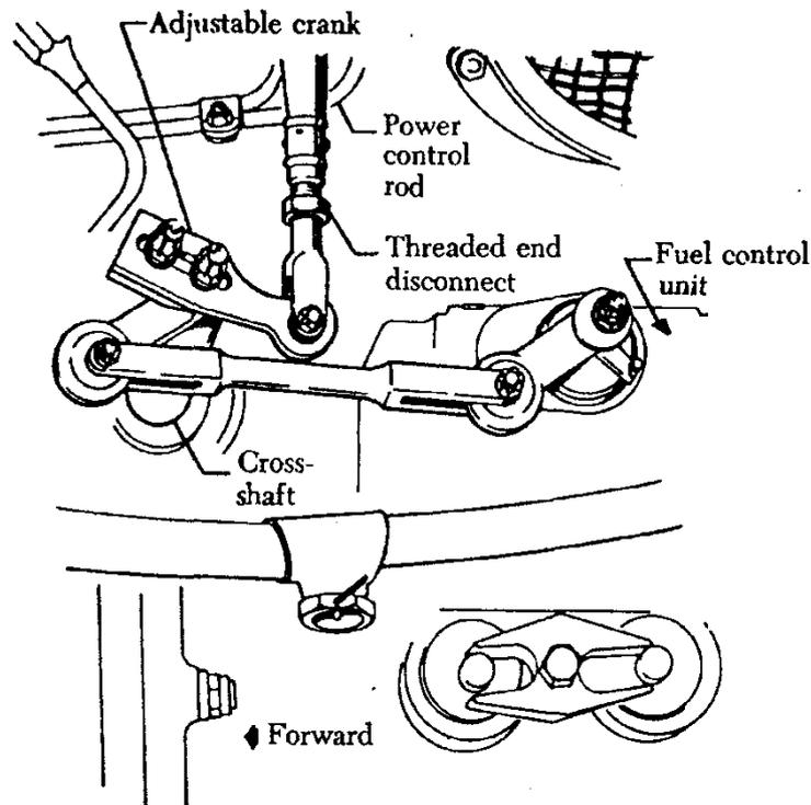
Gambar 32 Power lever disconnect.
