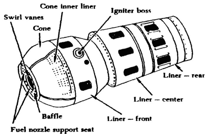
Gambar 37. combustion chamber liner nomenclature
