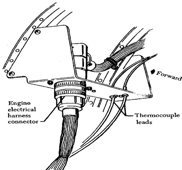
Gambar 30. Electrical disconnect
