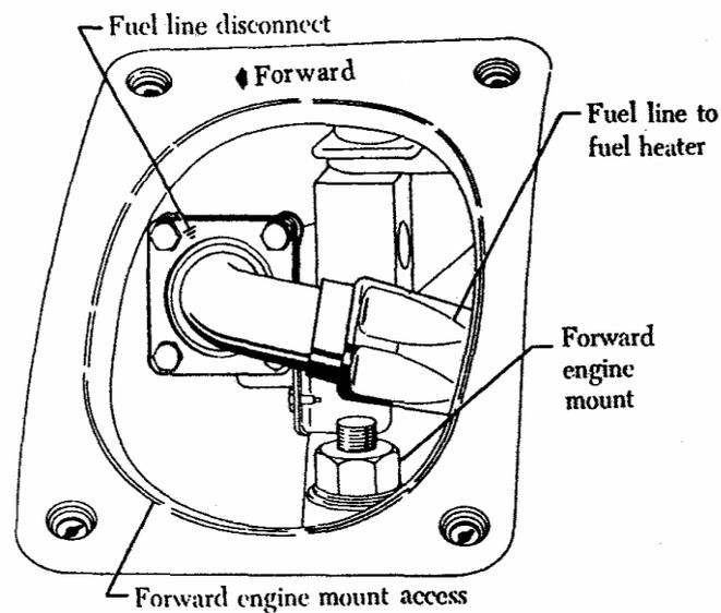
Gambar 31. Fuel line disconnect.
