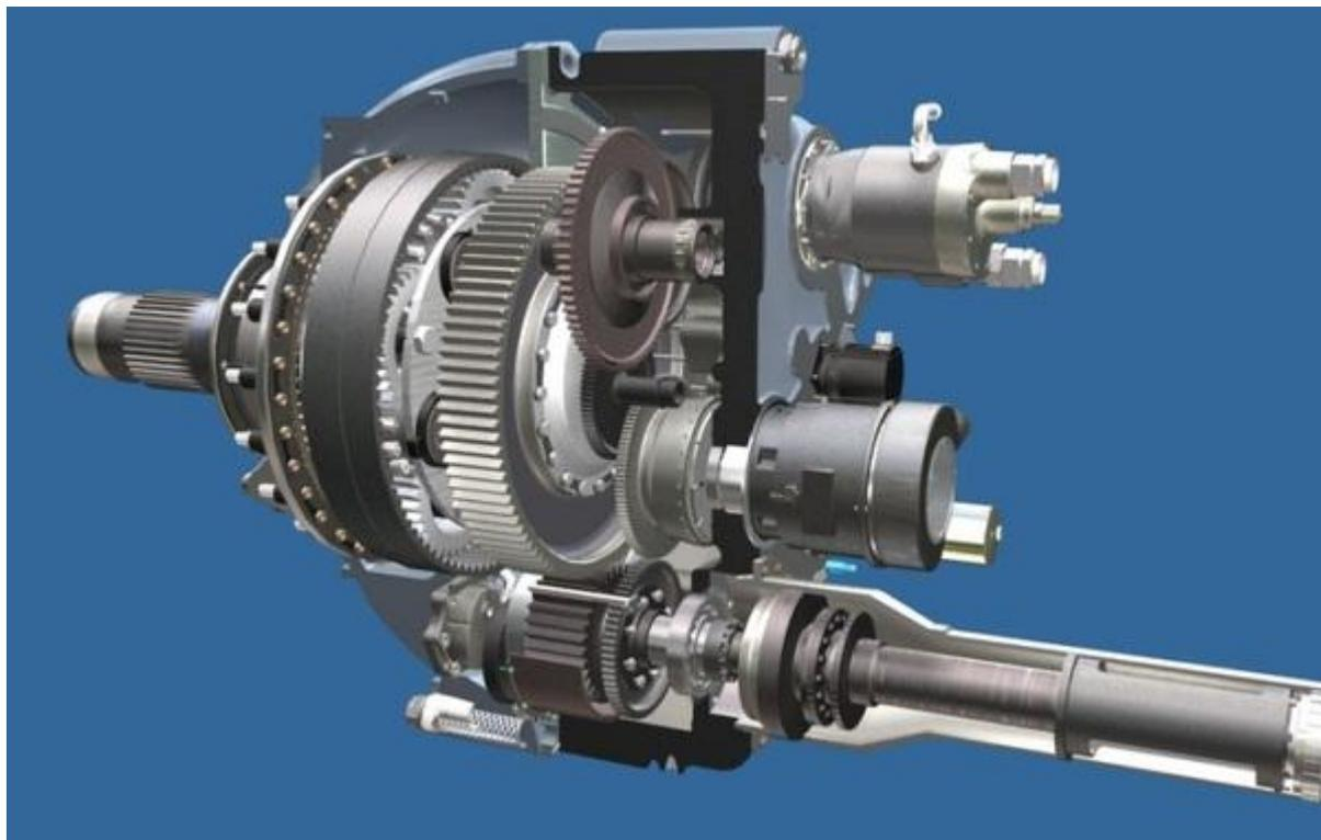
Gambar 8: T56-turboshaft Engine reduction gear
