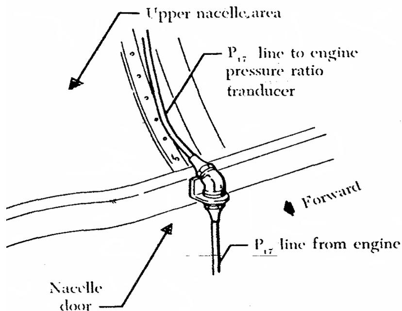
Gambar 29. turbine discharge pressure(Pt7)
