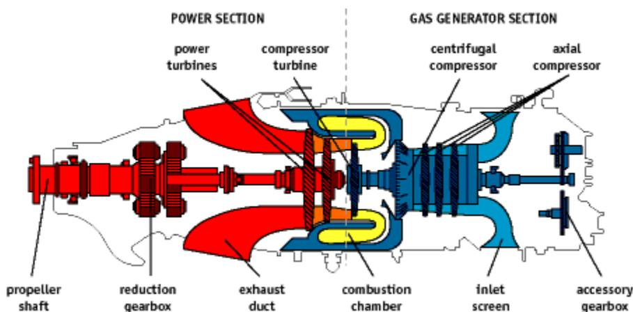
Gambar 6 :Reduction gear Turboprop engine
