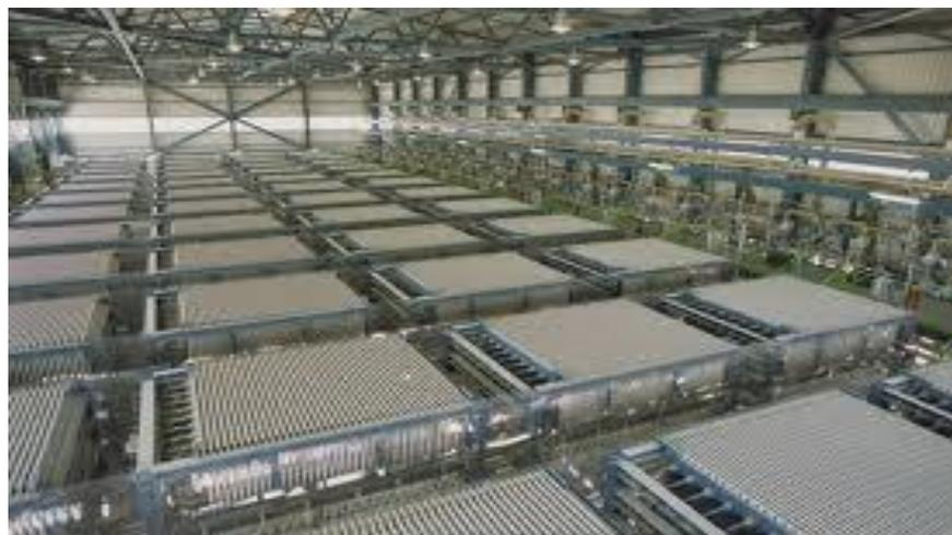
**Gambar 35. Proses Pembuaatan Gas Chlorine, Gas H<sub>2</sub> Dan Larutan Soda Kostik**
