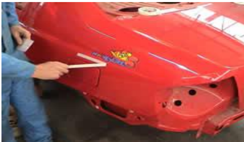
Gb.2.54. Pelepasan masking tape penanda
