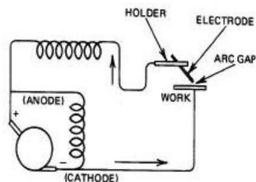
Fig. 1-4 Wiring Diagram, DCRP
