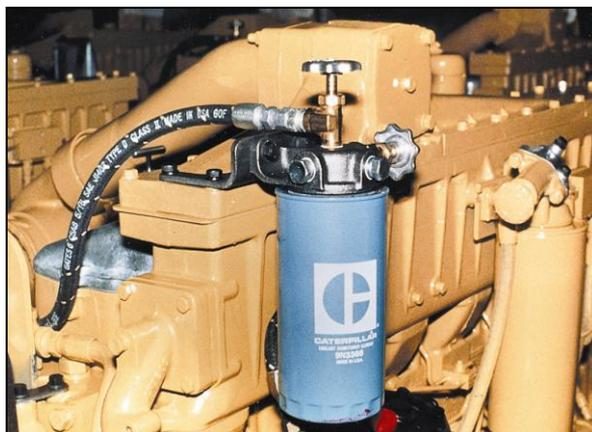
Gambar 2.15. Supplement coolant additive element
