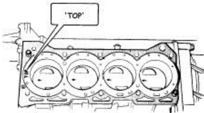
Gambar 3.160. Memasang gasket
