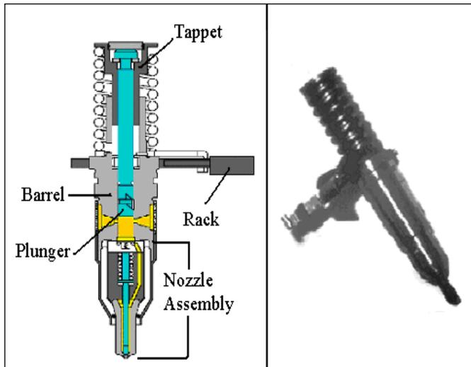
Gambar 2.53. Unit *Injector*
