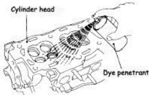
Gambar 3.135. *Dye Penetrant*
