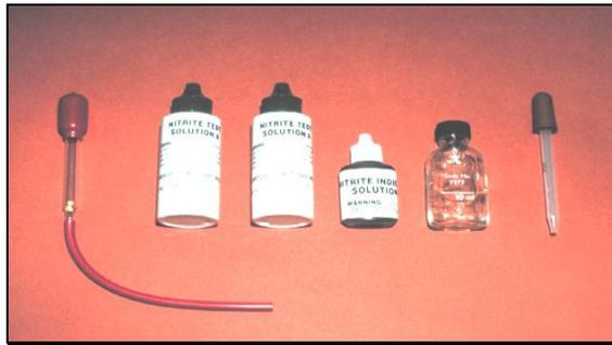
Gambar 2.18. Coolant conditioner test kit
