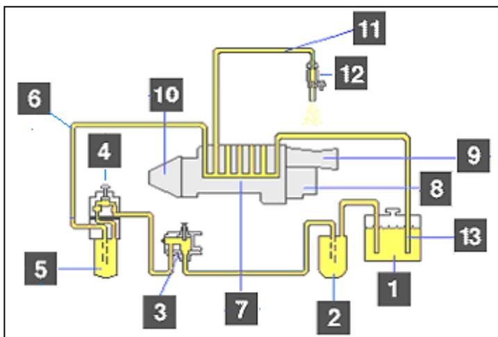
Gambar 2.39. Sistem Bahan bakar *Pump & Line*
