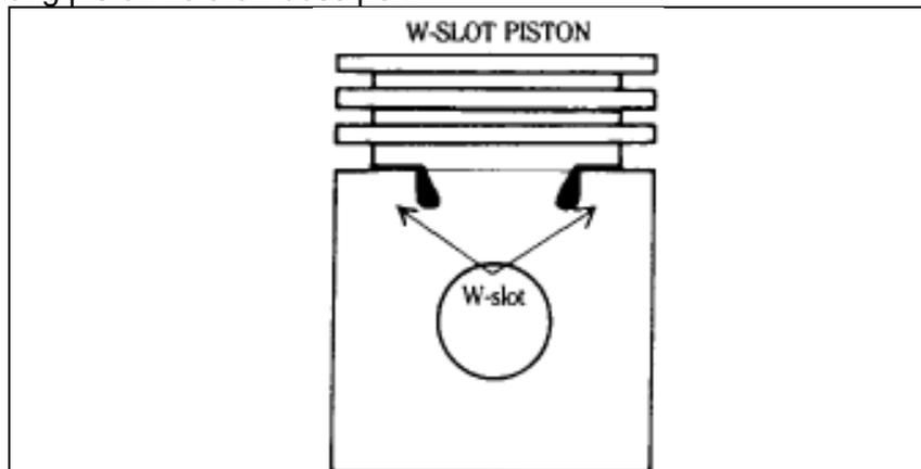
Gambar 3.64. Piston slot "W"
