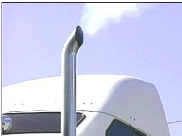
Gambar 1.24. *Exhaust Stack*
