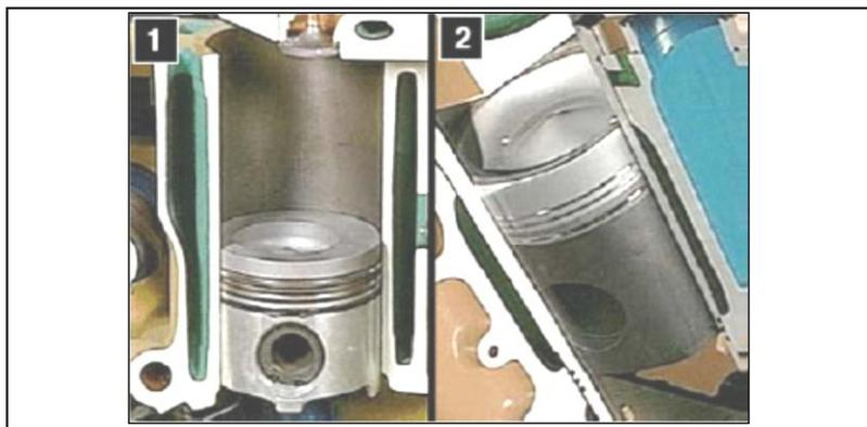
Gambar 3.58. *Cylinder liner*
