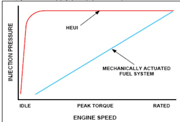
Gambar 2.61. Kurva Pengaturan *Hydraulic Injection Pressure*
