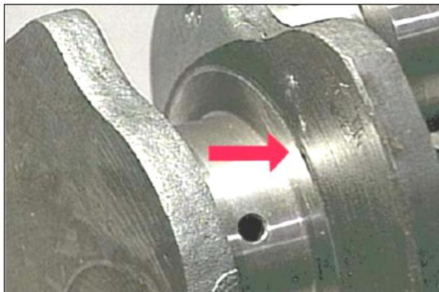
Gambar 3.104. Permukaan *Thrust Bearing*
