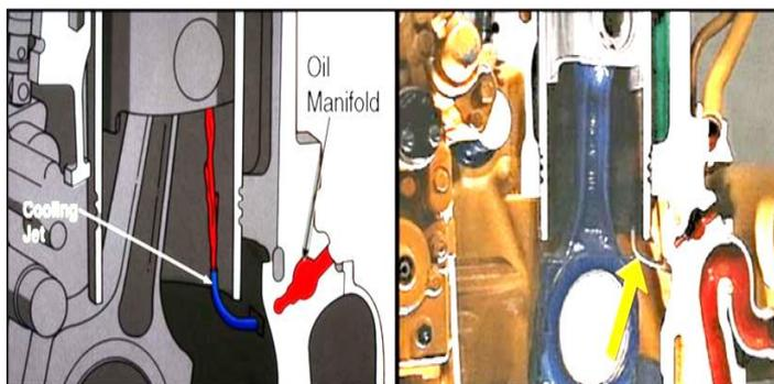
Gambar 2.28. Piston Cooling Jet
