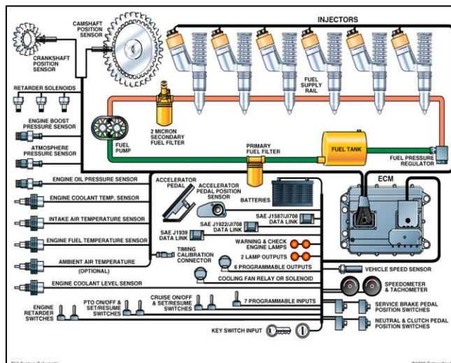
Gambar 2.55. Diagram sistem bahan bakar *electronic unit injector*
