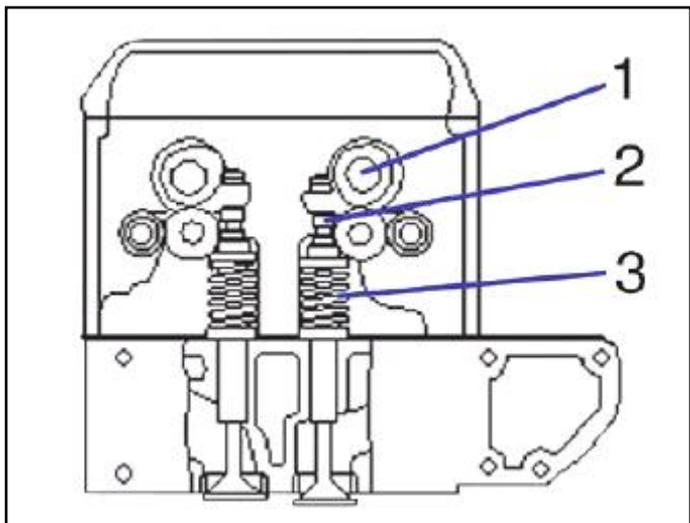
Gambar 3.170. Jenis over head cam shaft
