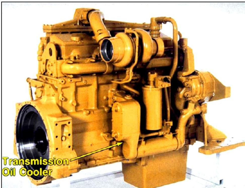
Gambar 3.129. *Transmission oil cooler*
