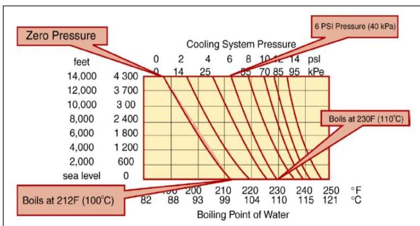
Gambar 2.13. Cooling sistem pressure & temperatur
