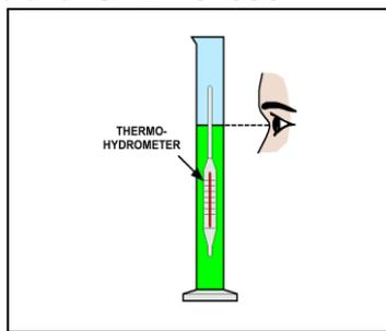
Gambar 2.62. Fuel Hydrometer
