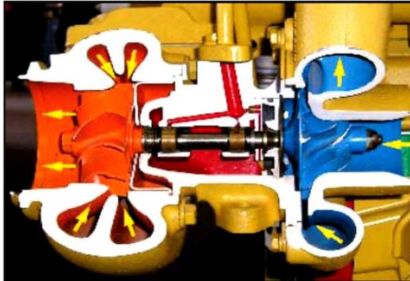
Gambar 1.22. Cara Kerja Turbocharger
