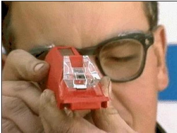
Gambar 2.19. Coolant & battery tester
