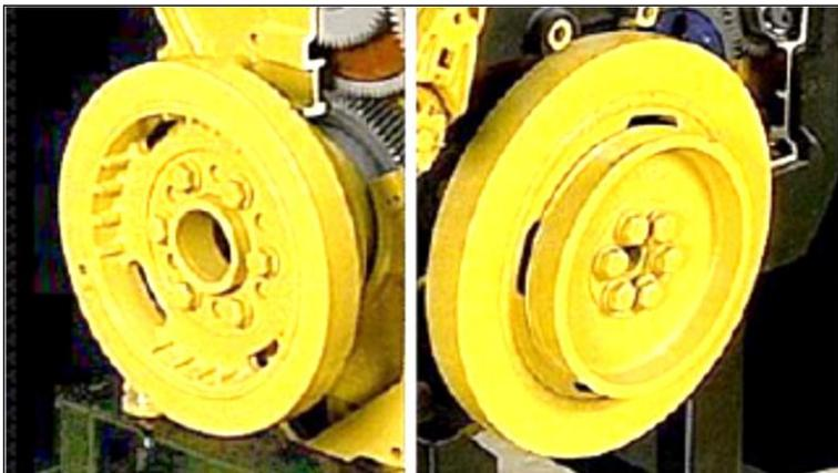
Gambar 3.106. *Rubber damper* dan *Viscous damper*
