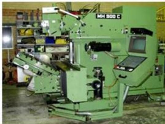
Gambar 4.23. Mesin Frais CNC
