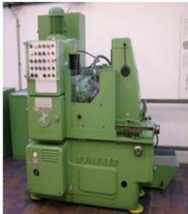
Gambar 4.21. Mesin Frais hobbing
