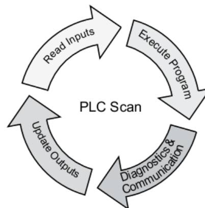
Gambar 4-21. Proses PLC scanning.
