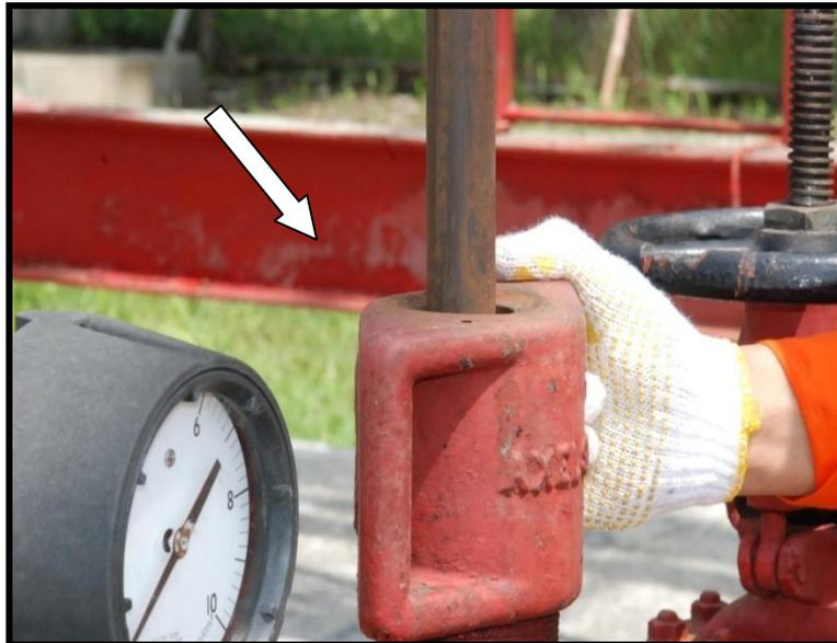
Gambar : 7.10 Mengecek stuffing dan polished rod
