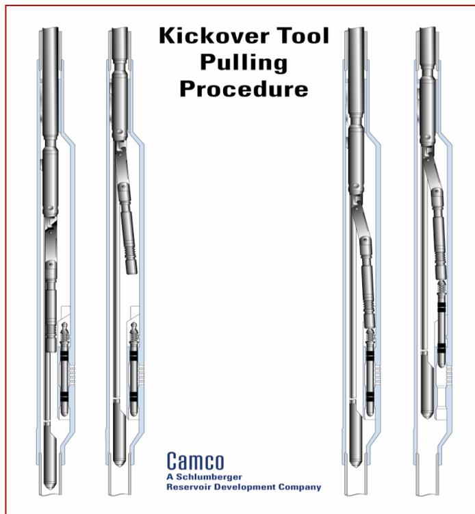
**Gambar 6-5 : Pulling Procedure**
