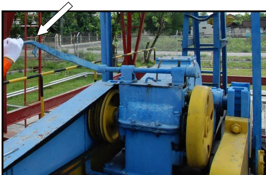
Gambar : 7.9 Mengecek Handbrake
