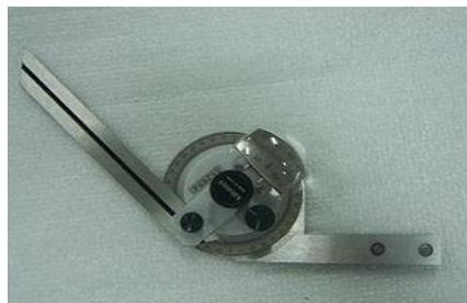
Gambar 5.32 Bevel protractor
