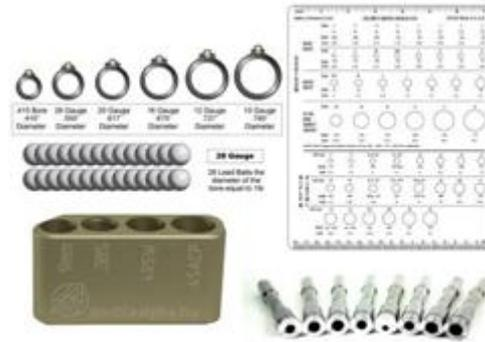
Gambar 2.10 Alat Ukur Kaliber
