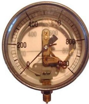
Gambar 5.20 Alat ukur *bourdon tube*
