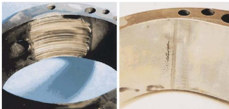
Gambar 4.39 Penampang cam ring (seizure, notched and erosion)
