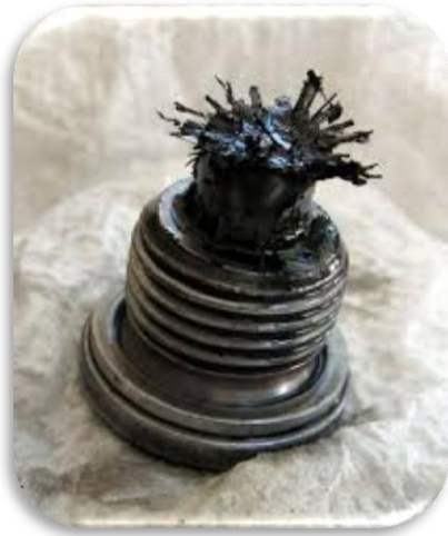
Gambar 3.8 Magnetic drain plug
