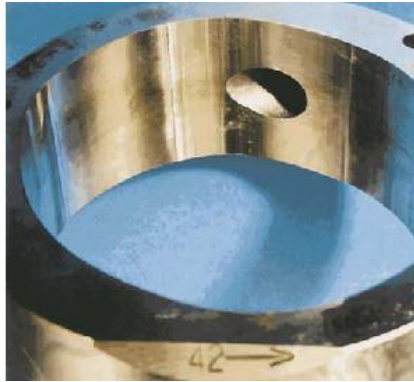
Gambar 4.37 Penampang cam ring (wear)
