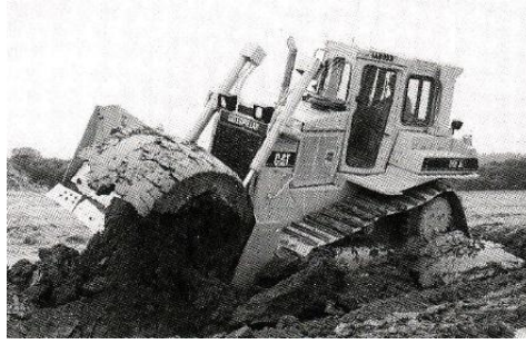
Gambar 6.2 Operasi dozer saat dozing
