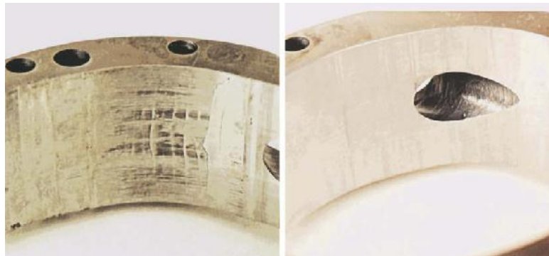
Gambar 4.40 Penampang cam ring (aerated, frosting and ripple)
