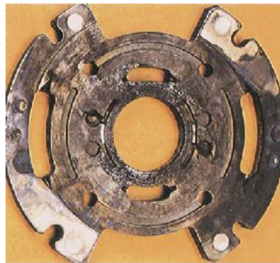
Gambar 4.35 Penampang flex plate (burn oil residu)
