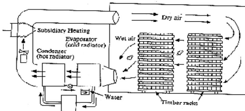
Gambar 3-5. Diagram *dehumidifier kiln dry*
