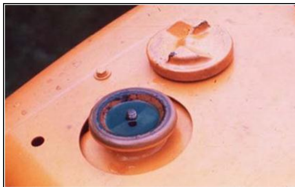
Gambar 10.107 Periksa level coolant
