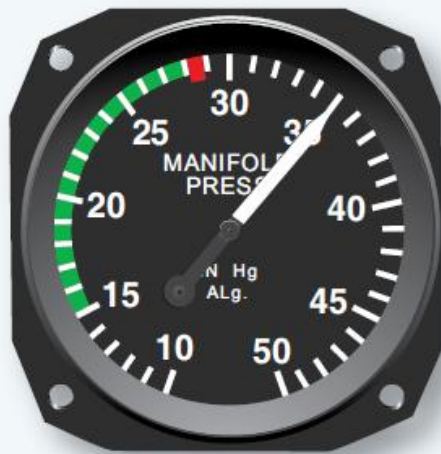
An analog manifold pressure indicator instrument dial calibrated in inches of mercury (left).
