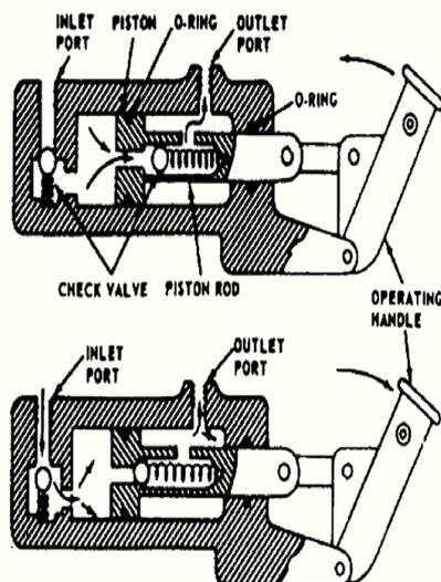
Gambar 4. *Hand Operated Hydraulics Pump*
