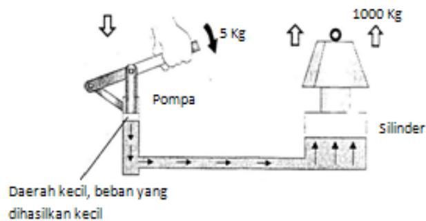
**Gambar 71. Prinsip Dongkrak Hidrolik**
