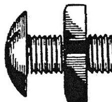
Gambar 133. Gutter Bolt
