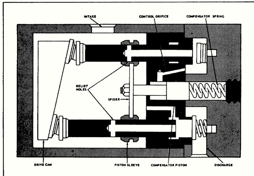
Gambar 9. Variable Delivery Piston Pump
