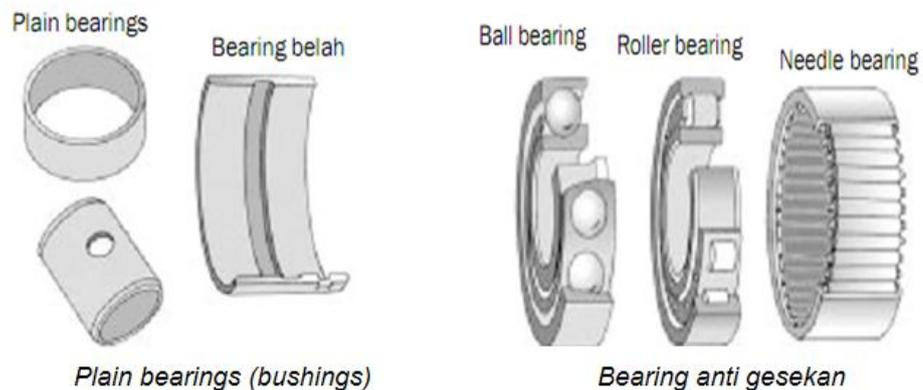
Gambar 24. Plain bearing dan roller bearing
