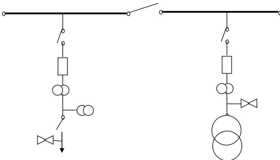
Gambar 2-5 : Single line diagram gardu induk single busbar
