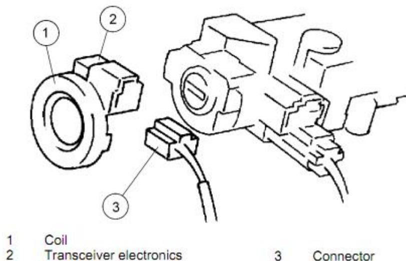
Gambar 9.7 Antena koil (*coil antenna*)
