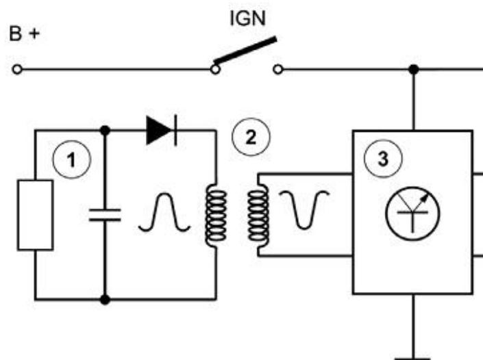
**Inductive coupling of transponder and coil antenna**
