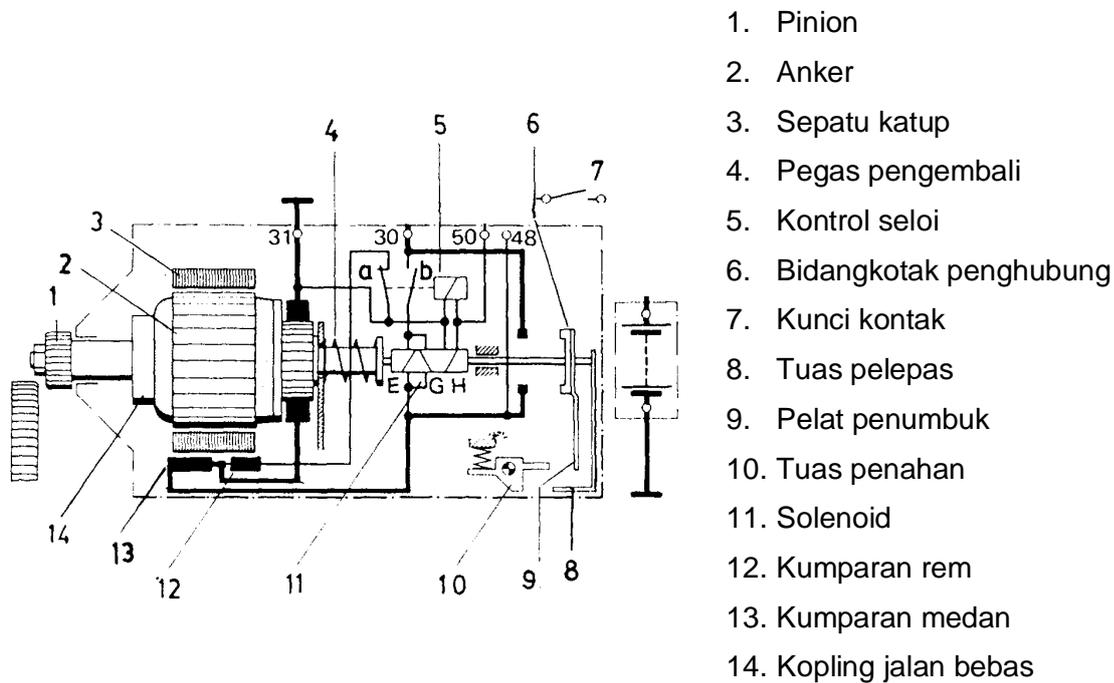
Gambar 6. 27. Skema stater batang dorong pinion
