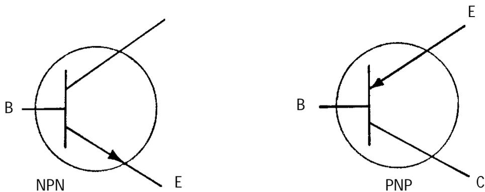
Gambar 5.34. Transistor
