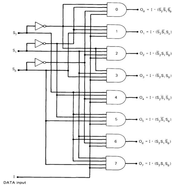
**Gambar 1.28 Rangkaian Logika 1 Line to 8 Line**
