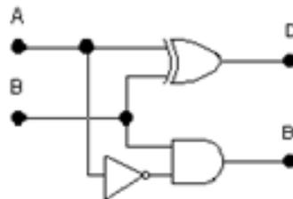
**Gambar 1.12 Rangkaian Half Subtractor**
