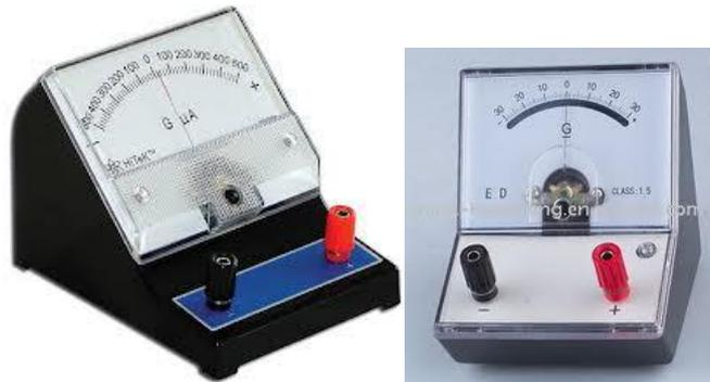
Gambar 6.9 Galvanometer
