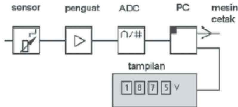
Gambar 6.4 Prinsip Alat Ukur Digital
