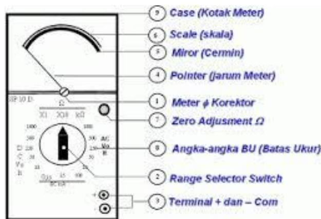
Gambar 8.3 Tipikal Multimeter
