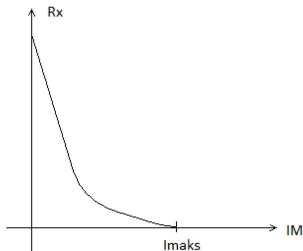
Gambar 8.5 Kurva Kalibrasi Ohmmeter Seri
