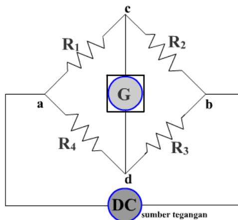
Jika  $R_1 \cdot R_3 = R_2 \cdot R_4$ , maka  $V_{cd} = 0$
