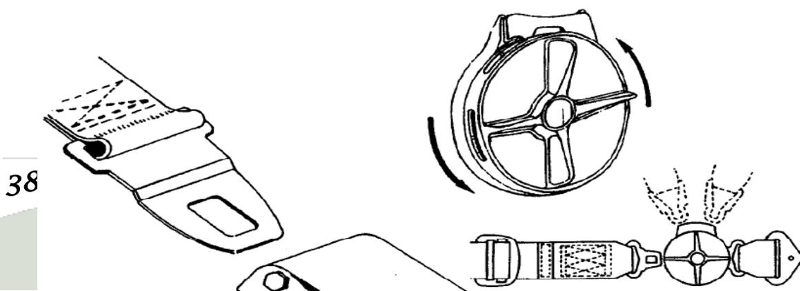
Gbr 6. Lift lever buckle dan rotary buckle
