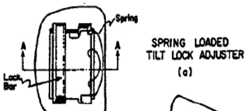
Gbr. 8 spring loaded tilt lock adjuster
