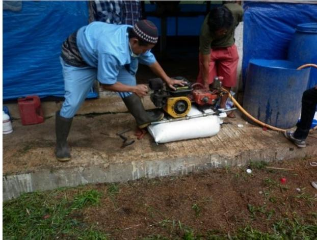
**Gambar 7. Cara mengoperasikan *Power Sprayer***
