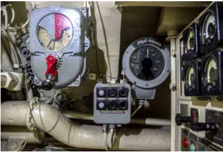
Alat Pengukur Kecepatan dan Arah Kapal Equipment to Measure Boat Speed and Orientation
